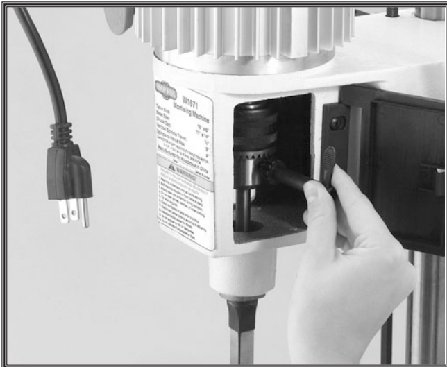
Figure 2. Unplug before changing chisels.
