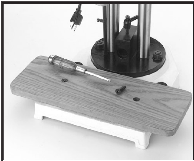
Figure 14. Work table secured with screws.
