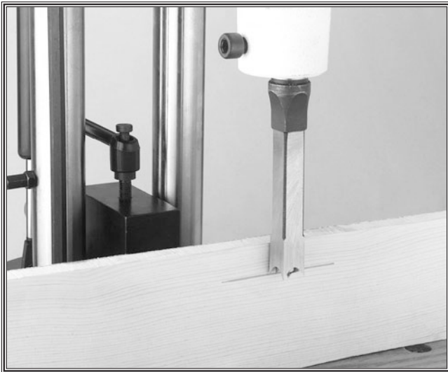
Figure 32. Use penciled line to gauge depth.
