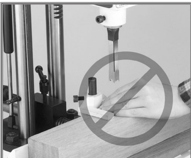
Figure 6. Never place hands under chisel.
