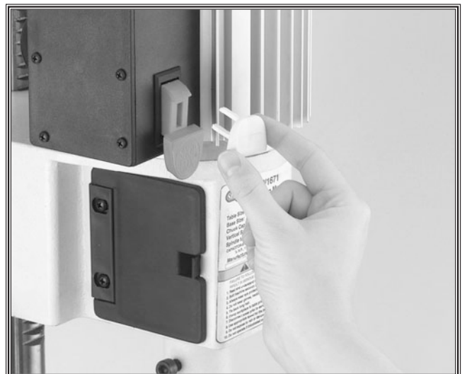
Figure 5. Remove safety key when not in use.
