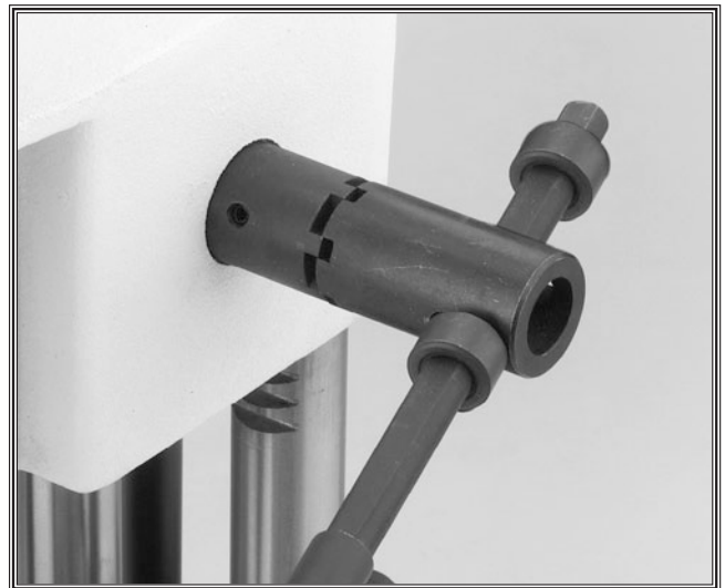
Figure 12. Indexing handle by swinging out.
