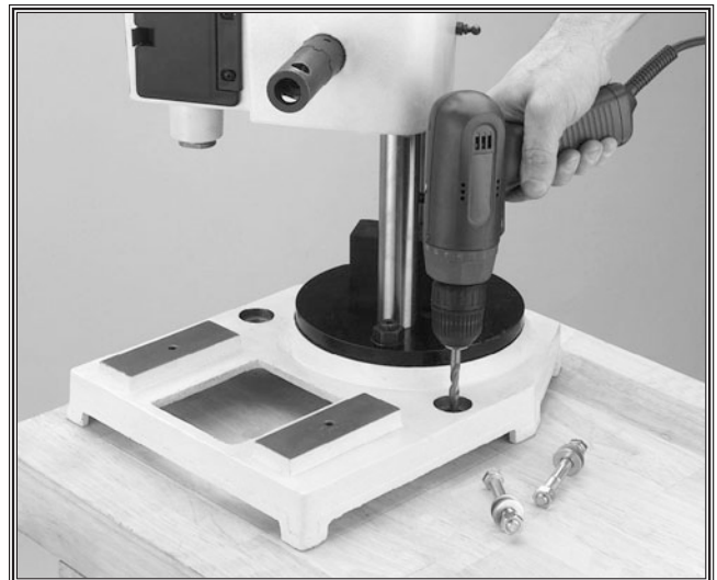
Figure 10. Using mounting holes as drill guides.
