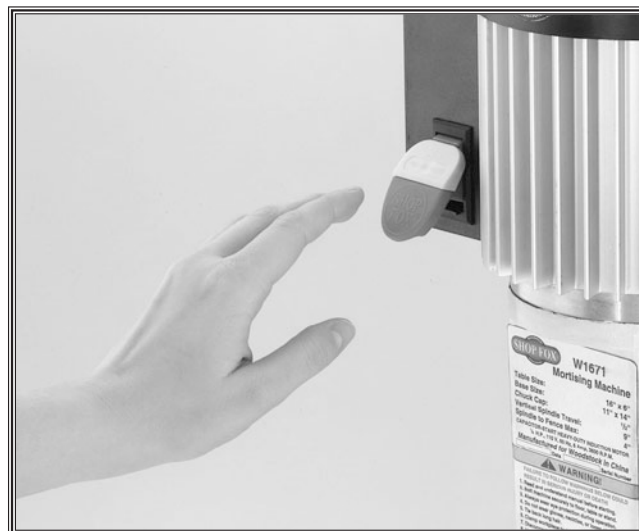
Figure 30. Hand poised over stop paddle.
