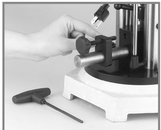
Figure 26. Setting micro-adjusting block.
