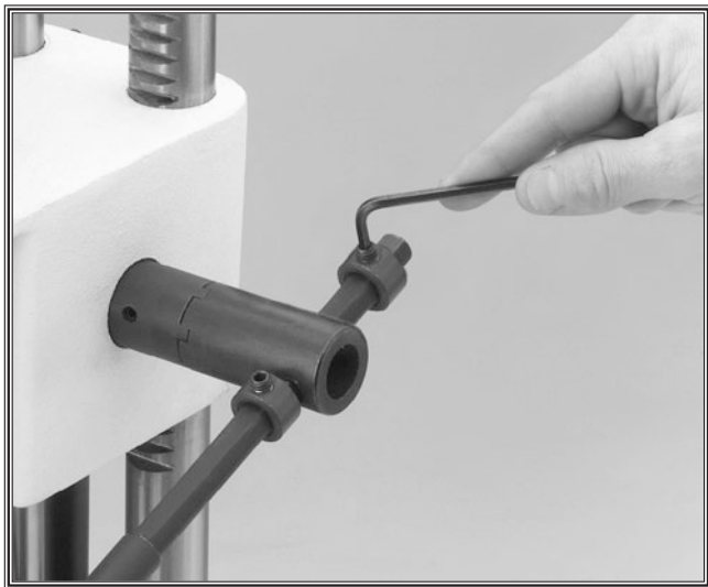
Figure 11A. Secure collar onto hand lever.
