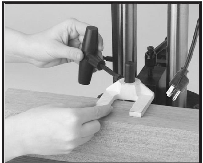
Figure 3. Always clamp workpiece.
